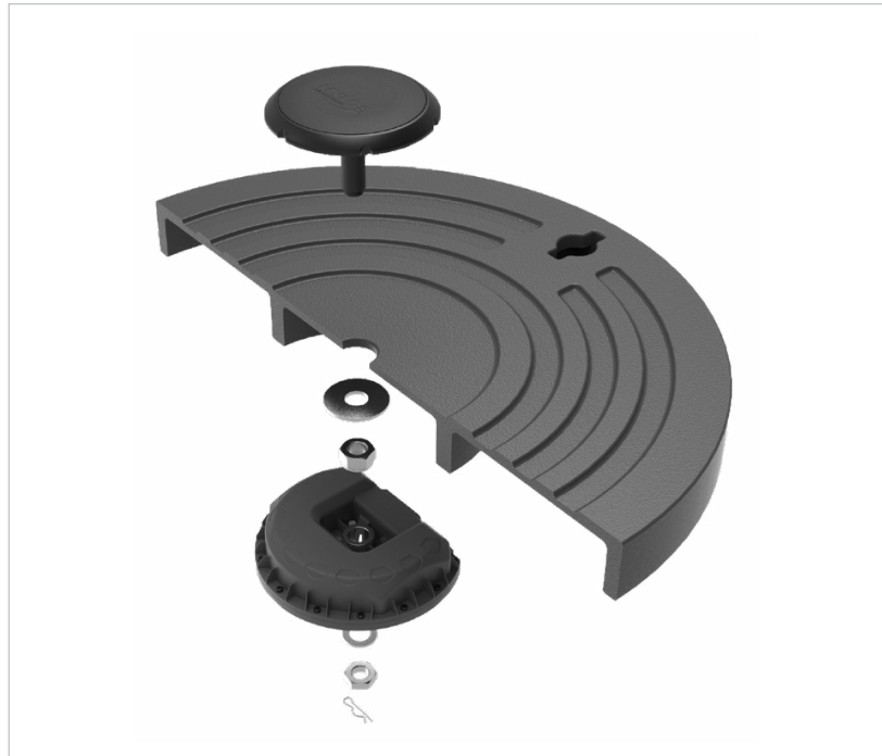
FIG. 1 Smarterwater® Stormwater Manhole Sensor Exploded Diagram
